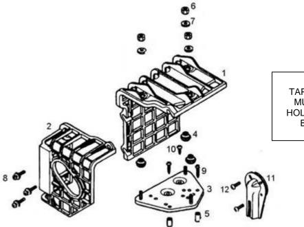
REMARK TAPPING SCREW (REF 9) MUST BE MOUNTED IN HOLES '2' MENTIONED ON BASE COMP.(REF 3)
