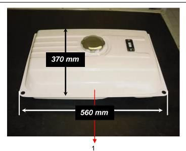
Height = 135 mm (measured without fuel filler cap comp. and fuel cock assy.)
